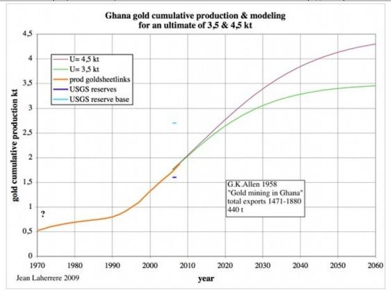
Figure 8: Ghana cumulative production & modelling for an ultimate of 3.5 & 4.5 kt Ghana's gold production should peak around 2015 at a level about 110 t/a.
