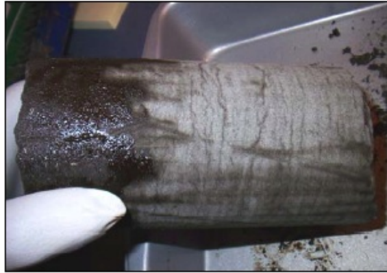
Figure 5. Whole round core sample of gas hydrate-bearing sand. Rind of oil-based mud coats the left end of the core.
