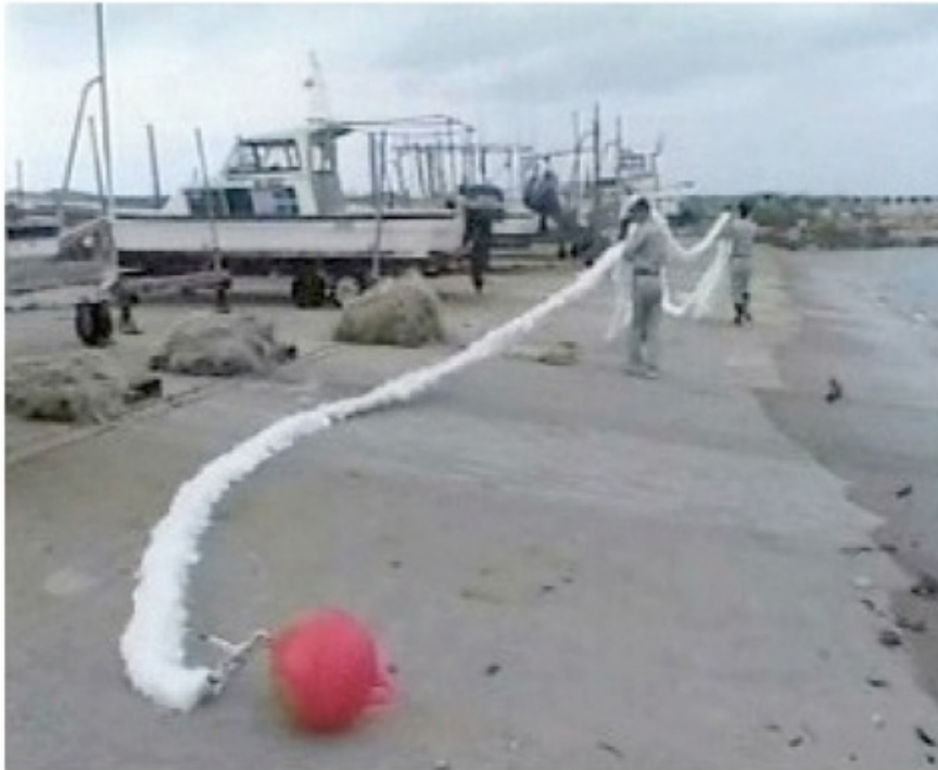
Figure: Japanese researchers testing uranium extraction from seawater using a braided adsorbent fiber (JAEA 2006). Is this the way of mining of the future?
