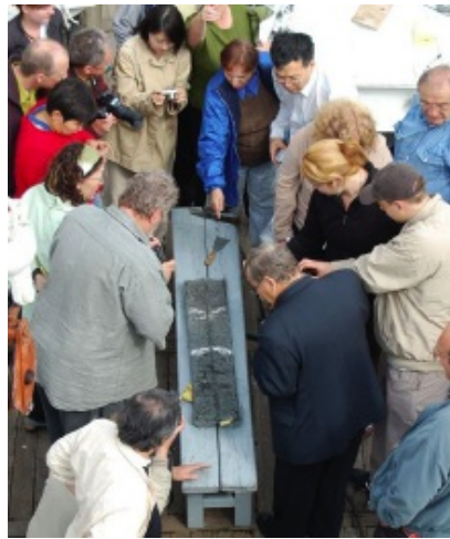
Figure 10 - A core drilled in September of 2007 in Lake Baikal showing two clear centrimetric hydrate layers.
