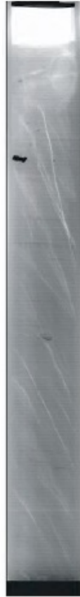
Figure 4: An example longitudinal X-ray image of a one-meter-long pressure core obtained from offshore India containing gas-hydrate bearing fractured clay-dominated sediments. Gas hydrate (lightest shading) occurs primarily as thin, high-angle features filling apparent fractures (photo courtesy of NGHP Expedition 01).
