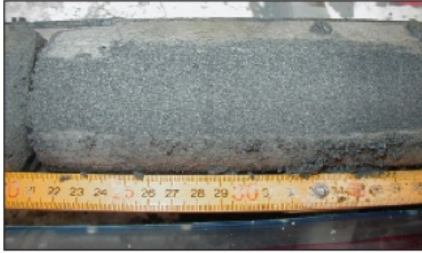
Example of disseminated gas hydrate (white specks) within porous and permeable marine sandstone from the Nankai Trough, offshore Japan (from Fujii, et al, 2005 ICGH Proceedings)
